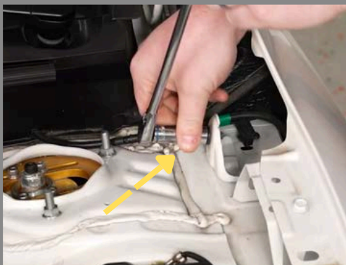
Step 6: Using a 12mm Socket, remove the Ball Stud from the Fender.
