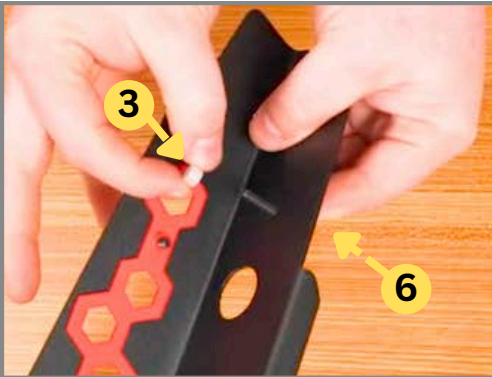
Step 2: Install Long 2.5mm Allen Bolt through the top of the Fender Shroud. Place Spacer on opposing side of Bolt.
