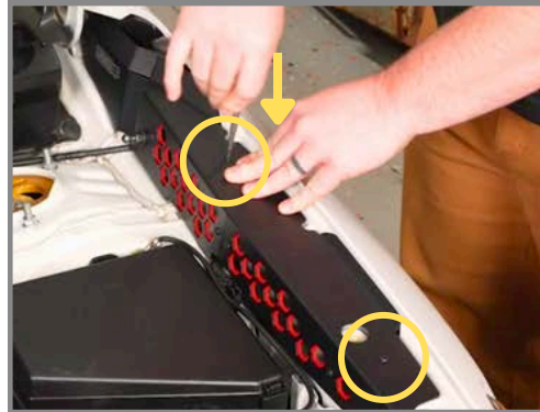
Step 9: Tighten the top Allen Bolts. Apply pressure to top of the Shroud to prevent the Riv-Nuts from spinning.
