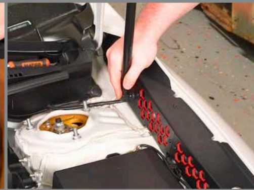
Step 10: Tighten the Ball Stud, then reinstall the Hood Strut. Repeat for other side.
