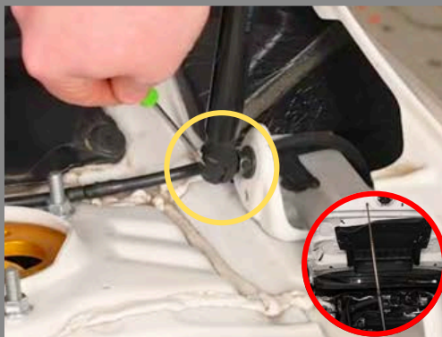
Step 5: Remove the Hood Strut from the bottom Ball Stud using a Screwdriver. NOTE: Support Hood using Prop Rod
