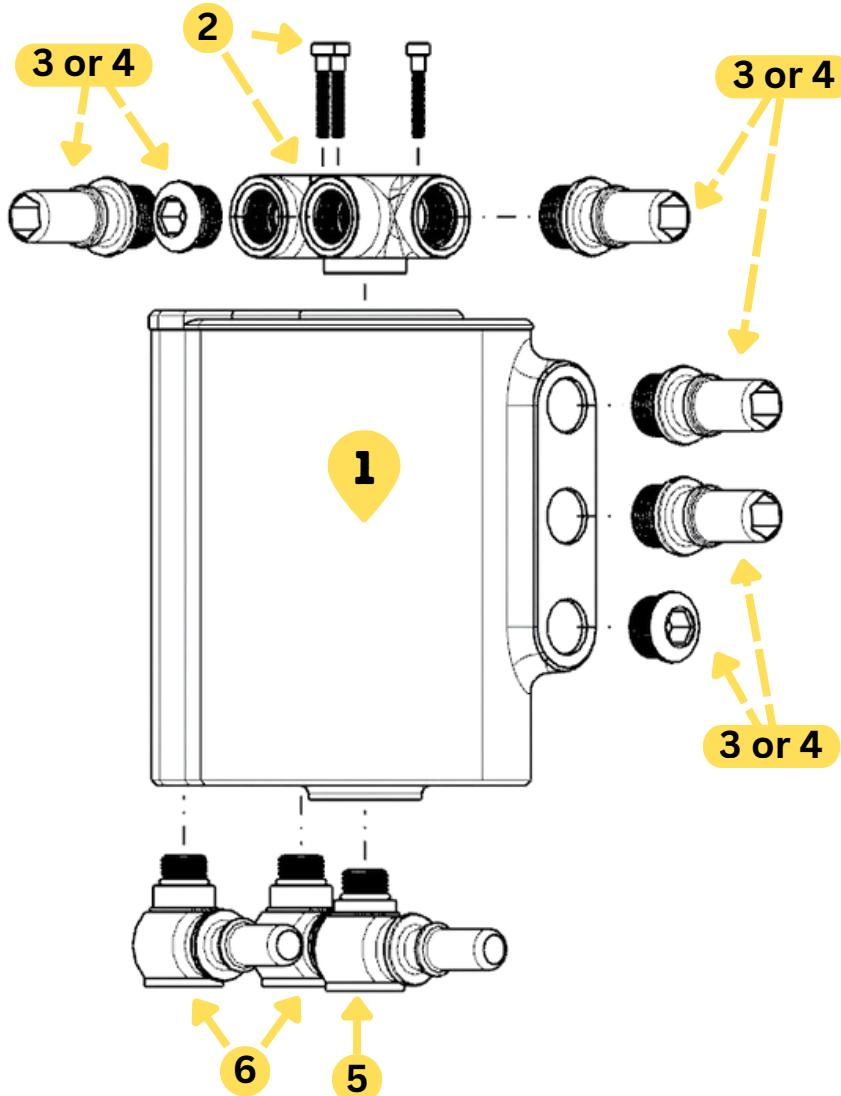
**Note:** Configuration of the Breather/Vent Ports may change based on vehicle. Use fittings or Block Offs as deemed necessary.
