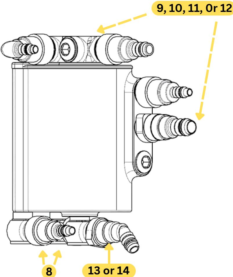
**Note:** Lubricate the O-Ring of ALL quick connect fittings with a synthetic multi-purpose grease to ensure a good seal.
